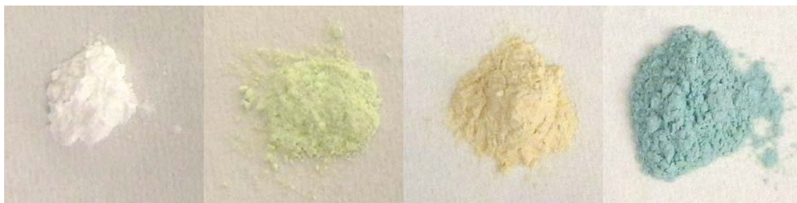
Figure 1. Colors of ZnO materials: white – pure, green – doped with Ni, yellow – doped with Mn, and blue – doped with Co.
